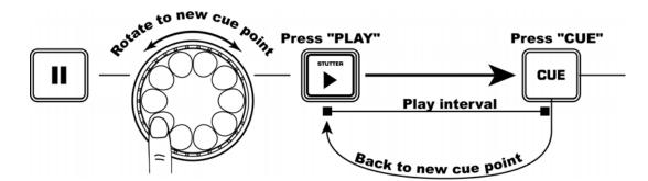
**EDITING CUE POINT:** When the jog wheel is turned while paused, a new cue point can be located. By pressing "PLAY" while paused that point will be set. By pressing "PLAY" again (STUTTER) the point can be checked as desirable.
